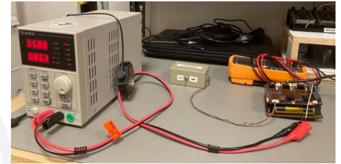
Flight Battery test – charging the battery with non-flight P31us.
